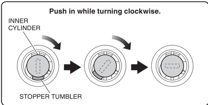
21. Draw out the key and check that the inner cylinder does not come out.
