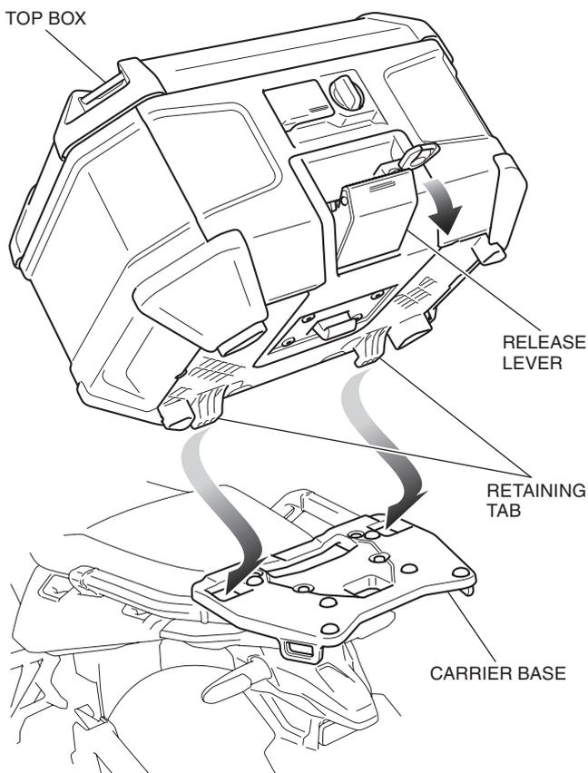
4. Position the hook of the top box on the carrier base as shown.
