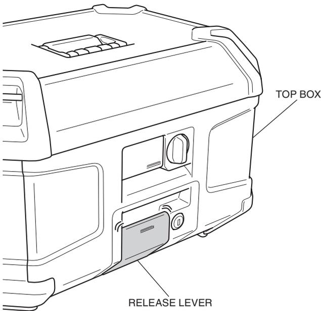
8. Check that the top box is installed securely by swinging the top box taking care not to fall the motorcycle down.
