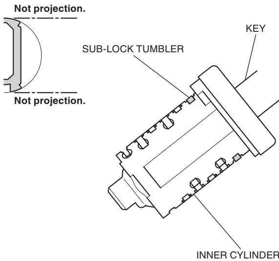
14. Insert the assembled inner cylinder into the body as shown.
