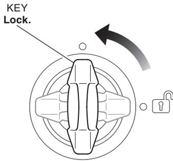
7. Remove the key. Be sure that release lever cannot be released.
