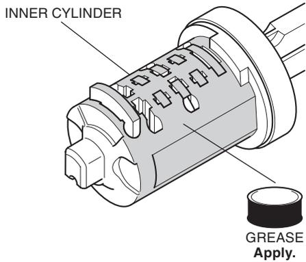
20. Install the inner cylinder by sliding the stopper tumbler along the slide guide while rotating it.
