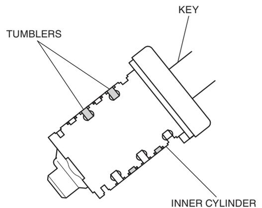
10. Install the tumblers and springs (silver) to the reverse side inner cylinder as shown.
