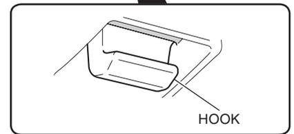
5. Secure the hook by push the release lever as shown.
